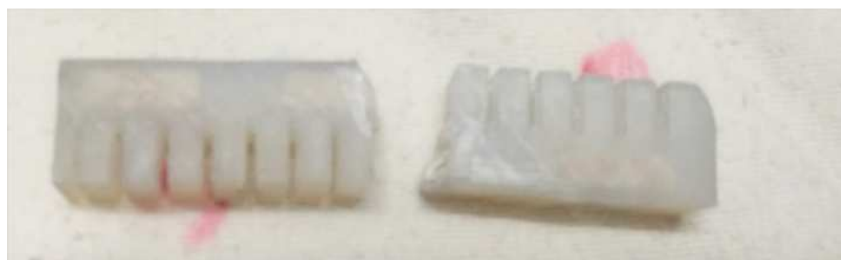
Figure 13: Breakage of Soft Finger
